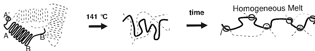
Figure 4: Depicting the melting process of the disentangled nascent crystals during fast heating. Upon fast heating the chains are likely to get mixed, leading to a gradual increase in the storage modulus with the formation of, ultimately resulting into a homogenous distribution of the entanglements in the melt.
