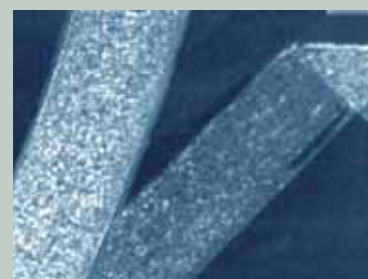
Nucleated Akulon® PA6 film (right) shows finer, denser crystalline structure compared to un-nucleated (left).
