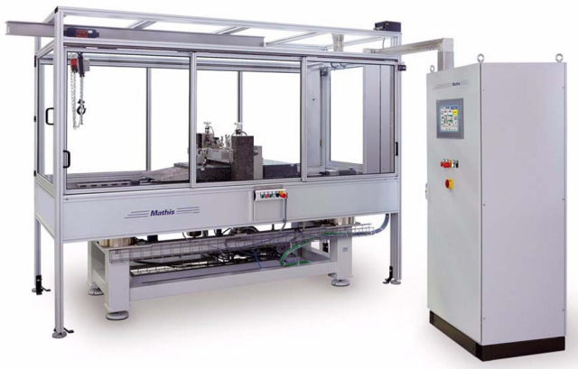
Figure 4. Slot-die coating process as developed by DSM.
