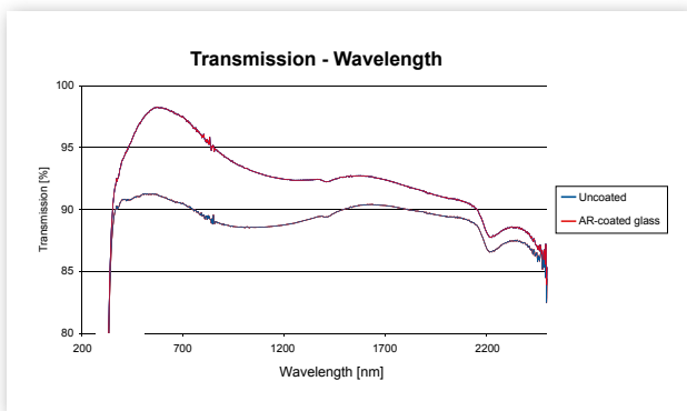
Figure 4: Comparing the transmission spectrum of double-sided KhepriCoat™-coated and uncoated 4mm low-iron float glass.
