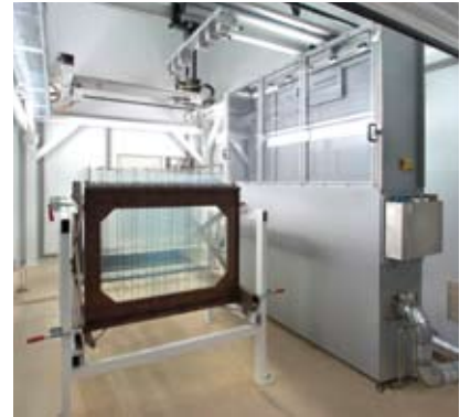
Figure 7: DSM's dip-coat unit is capable of dipping four glass sheets simultaneously
