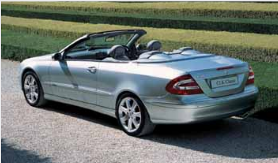
The new Mercedes CLK convertible has a Class A SMC decklid (picture DaimlerChrysler)
