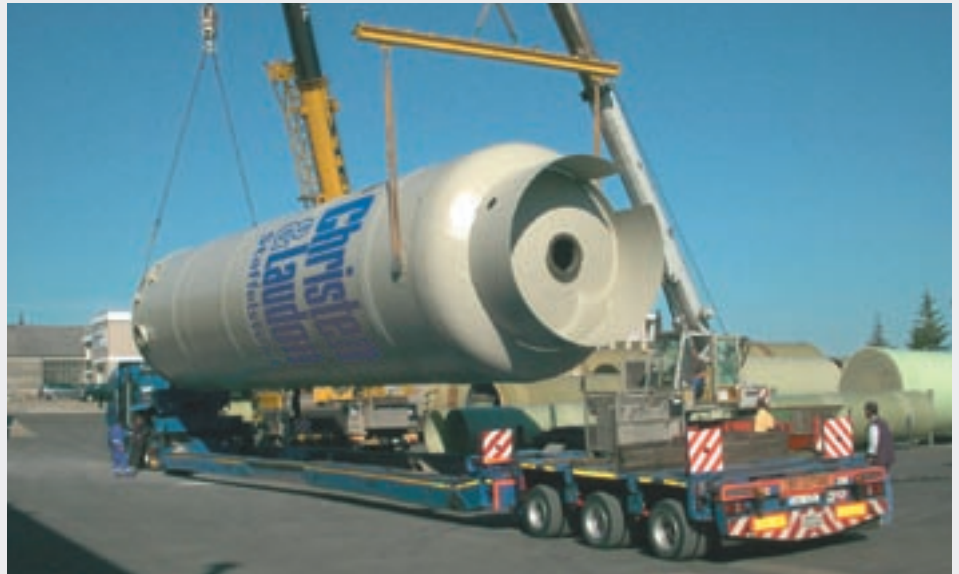
Chlorine dioxide storage tank based on Atlac 430 ready for transport
