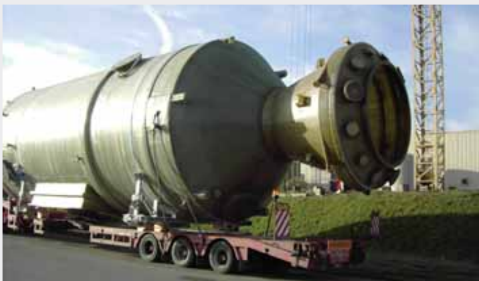
Atlac E-Nova FW 2045 and Atlac 430 used in a quench and scrubber
