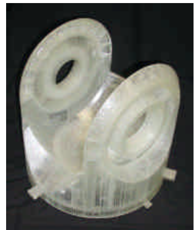
Somos WaterShed® 11120 produces highly accurate and stable investment casting patterns
