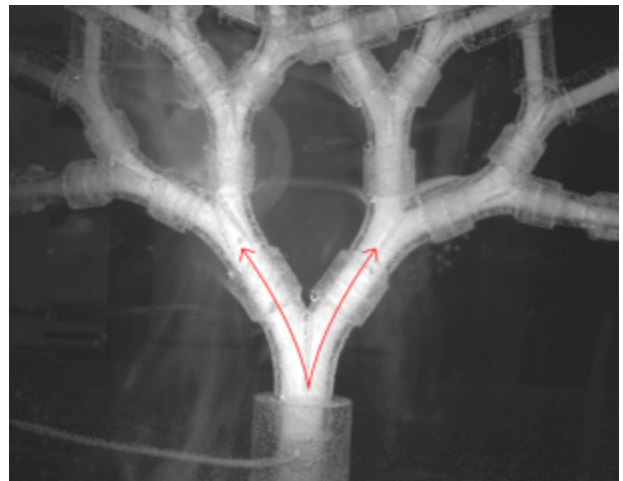
Above: A stereolithography model of a human lung made out of Somos WaterShed® 11120 highlights fluid flow in order to help predict behavior of particles entering the lungs.
