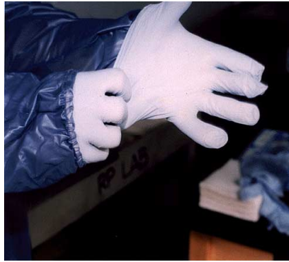
4. Don a second pair of nitrile gloves, pulling glove cuff over the oversleeve elastic gather.
