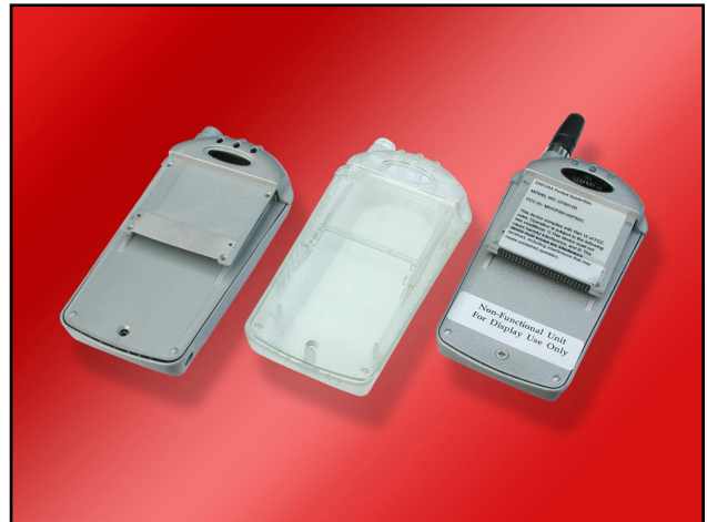
The Pocket Spider IIc, a small, compact wireless modem for PDA's designed by RP Innovations, Inc. for ENFORA, Inc. The Pocket Spider IIc was prototyped using unique DSM Somos® WaterClear™ 10120 – a new stereolithography resin providing the optical clarity of many polycarbonates.
