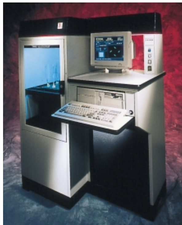
At the Centre for Rapid Design and Manufacture (CRDM), a single 250 mW laser beam was successfully split between two separate SLA®-250 machines, achieving two beams each capable of outputting 125 mW. (Photo courtesy of 3D Systems, Inc.)
