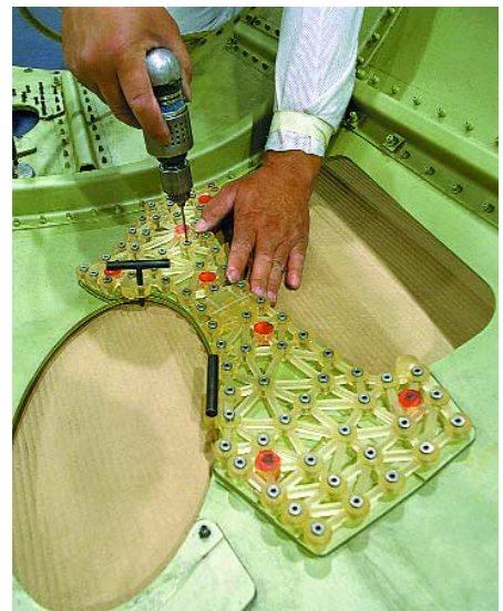
Northrop Grumman engineers use RMSTs made from Somos 8110 in the assembly of fighter jets.
