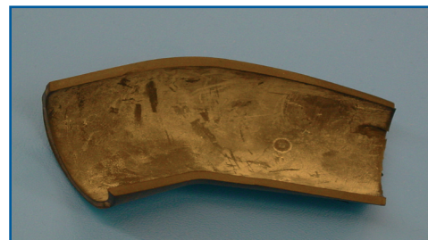
Figure 1: blooming on the surface of a profile.
