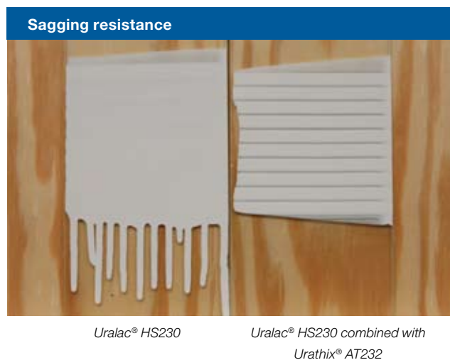
Figure 2: When applying thick layers of paint, the tendency to sag can be greatly reduced by using either the medium gel-strength thixotropic resin Urathix® AT231 on its own, or the Uralac® HS230 combined with the high gel-strength thixotropic resin Urathix® AT232.
