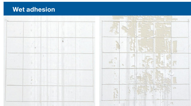
Figure 2: Neopac® E-128 (left) shows very good wet adhesion on old non-sanded alkyd substrate in comparison to a standard waterborne acrylic (right).
