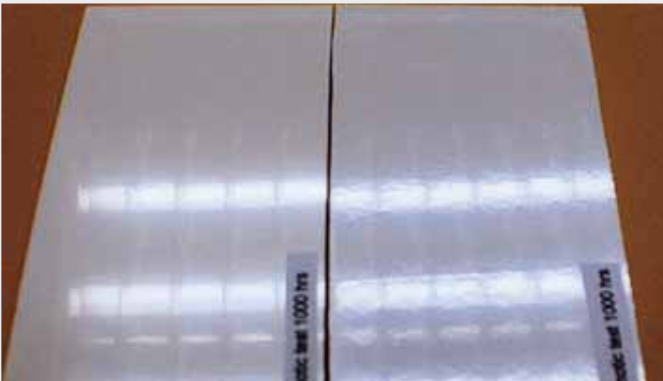
Superior surface profile of Neogel Eco/Atlac 580 (left) after 1000 hours intensive blister testing
