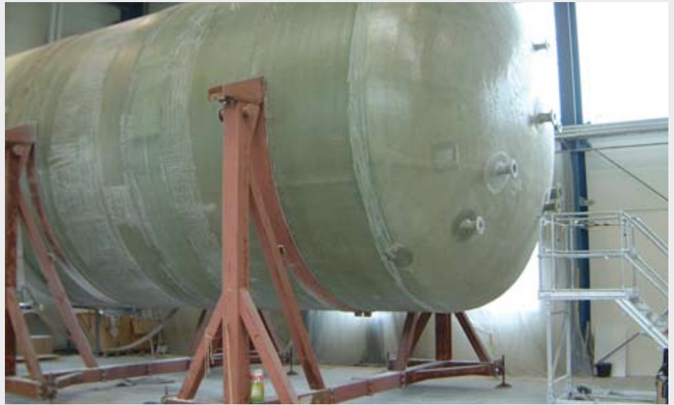
Production of Atlac storage tank for sodium hydroxide
