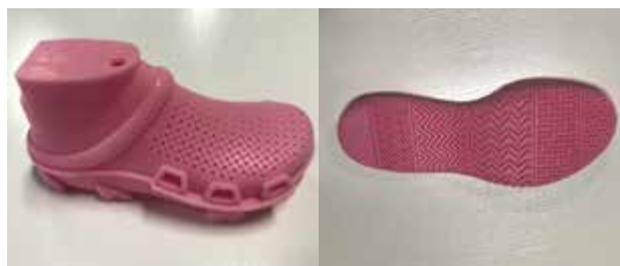
Other properties of Somos® Momentum that have helped to improve pattern mold development are dimensional stability and the ability to hold fine detail. The pink color of Somos® Momentum helps make the material easy to work with and quality check.
