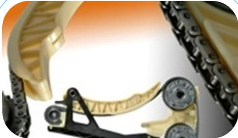
Chain tensioner in car engines, made from Stanyl<sup>®</sup>, gives higher durability, lowers weight & friction and saves fuel and CO<sub>2</sub> emissions
