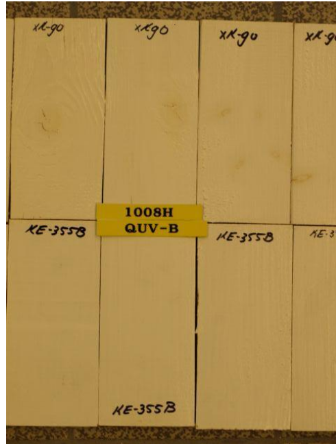
Figure 2. The anti-knot bleeding results of a system based on NeoCryl XK-90 (top) and SOP1 (bottom) after 1008 hours QUV (42 days).
