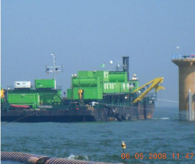
The four ropes used on this project were manufactured by BEXCO (Belgium). Each 500-meter length of rope had a MBL of 199mt. These ropes were used to moor the barge with four anchors to the seabed. They are directly wound on the hydraulically operated and GPS-controlled traction winches.
