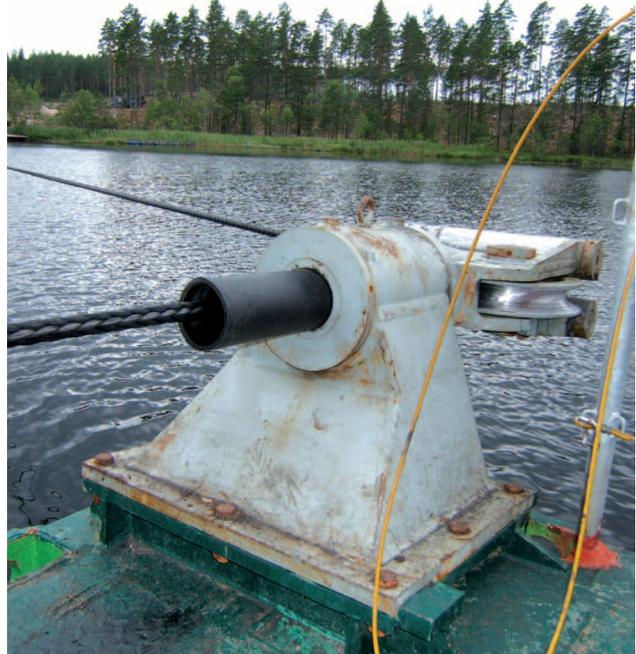
replacement, typically needed for SWR and other, less durable synthetic lines. Jorne Beyen noted, “during the use of the ropes only minor abrasion could be observed. This contributes to their long life.”
