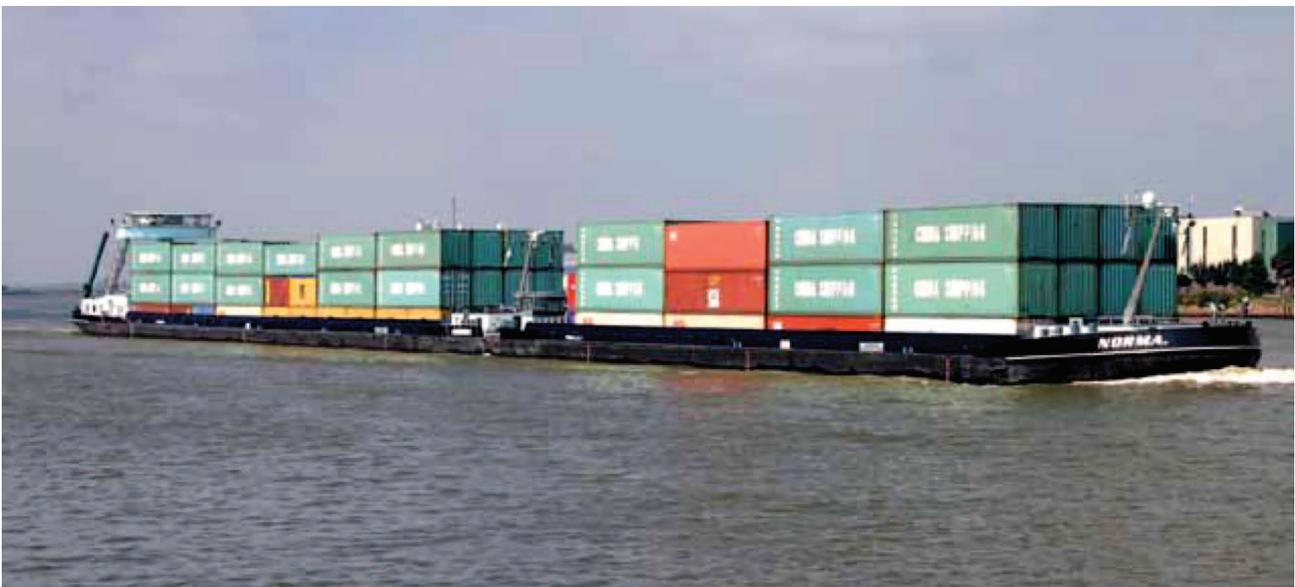
Push combination ‘Norma’ has been in service since July 2007. From its maiden voyage onwards, four Eurolest® ropes with Dyneema® manufactured by Lankhorst Ropes have been used onboard. The purpose of these ropes is to connect the vessel to the barge being pushed. Captain Grinwis and his crew – all of whom have had a lot of previous experience with SWR on other push combinations - are extremely
