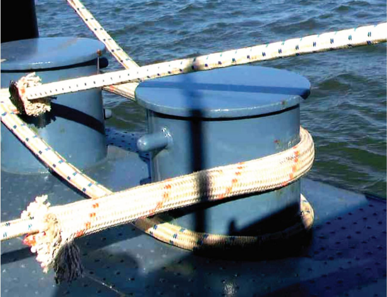
The ropes are equipped with a highly abrasion resistant cover made from Dyneema®, ensuring a reliable and durable solution following previous issues with the original polyester jacket.
