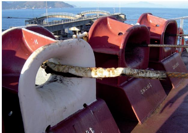
*Fairlead used for the passage of cables during the period the vessel is in the pier.*
