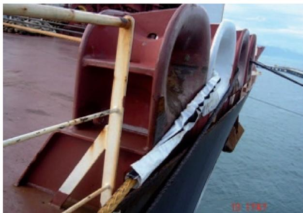
*Special protection for the cable with Dyneema®.*
