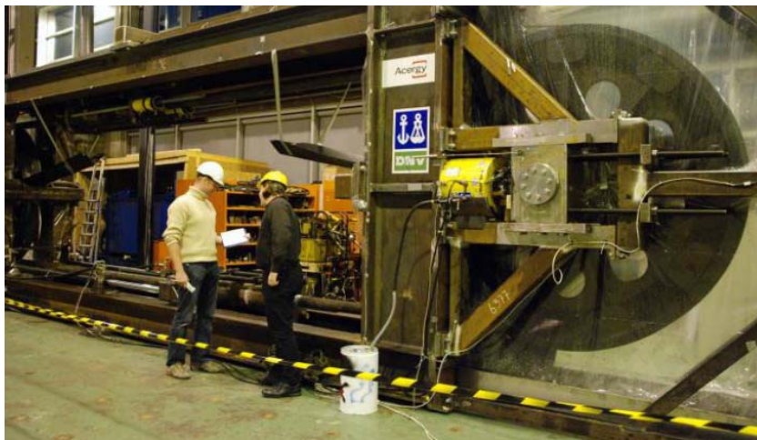
Figure 2: CBOS test rig at DNV Høvik, Oslo (Left). Sheave groove detail (Right)
