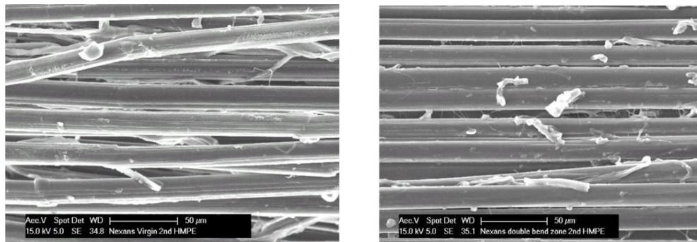
(B) Outer layer in virgin improved tether cable specimen (left) and CBOS tested (4,200 cycles) specimen (right).
