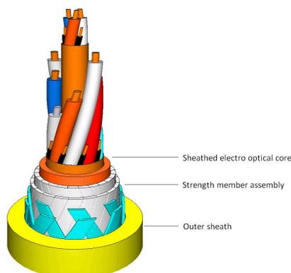
**Figure 2.** A three dimensional impression of the improved ROV tether cable design.
