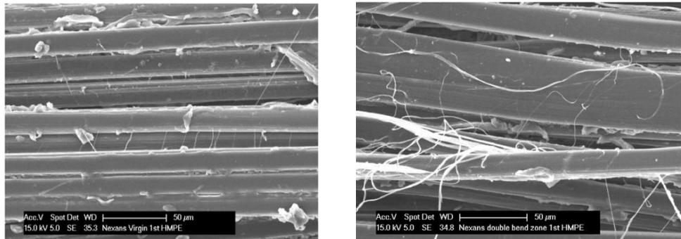
(A) Inner layer in virgin improved tether cable specimen (left) and CBOS tested (4,200 cycles) specimen (right).
