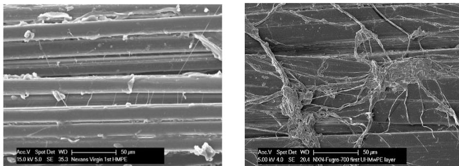
(A) Inner layer in virgin improved ROV tether cable specimen (left) and field tested specimen (right).
