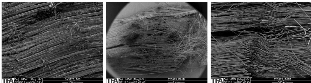
**Figure 1.** Impressions of internal abrasion (*left*), misalignment (*middle*) and compressive failures (*right*) of the strength member made with aramid fibers from an actual ROV tether cable.
