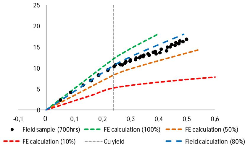
**Figure 4.** Axial stiffness measurement of field-tested improved ROV tether cable.
