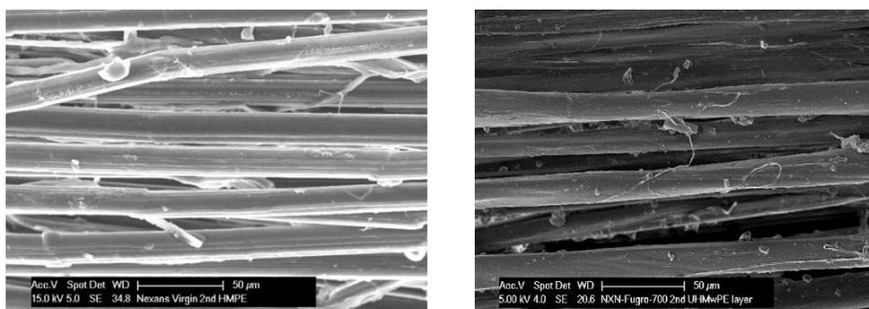
(B) Outer layer in virgin improved ROV tether cable specimen (left) and field tested specimen (right).
