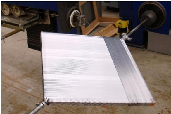
Figure 3. The winding specimen, here with Dyneema® fibers only
