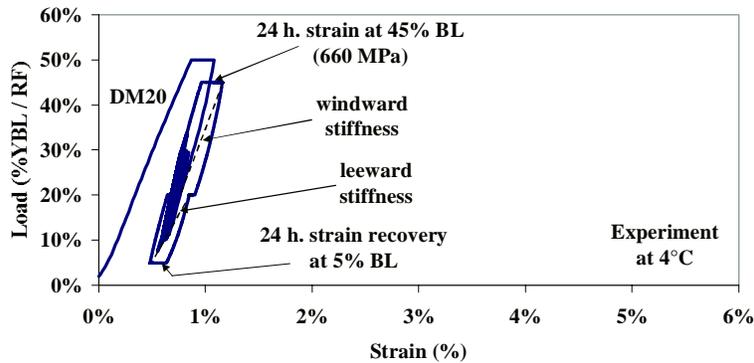
Figure 11. Load – strain results on DM20 fiber at 4°C, based on typical rope application realization factor
