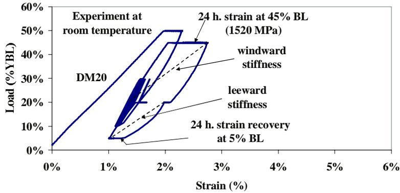
Figure 6. Load – strain results measured on DM20 fiber at room temperature, based on Yarn Break Load
