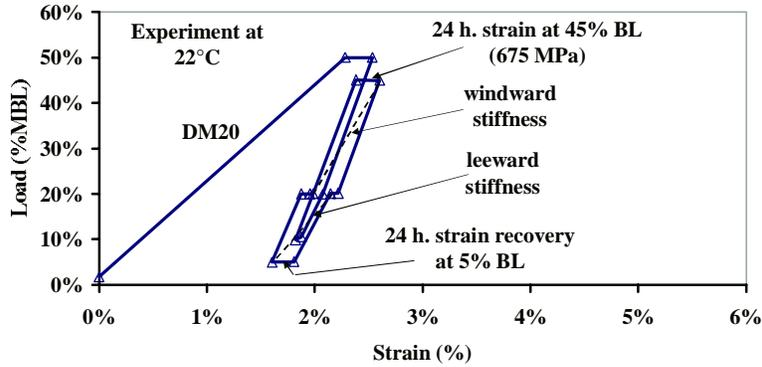
Figure 8. Load – strain results measured on 52 mm diameter subrope with DM20 fiber at 22°C [12]
