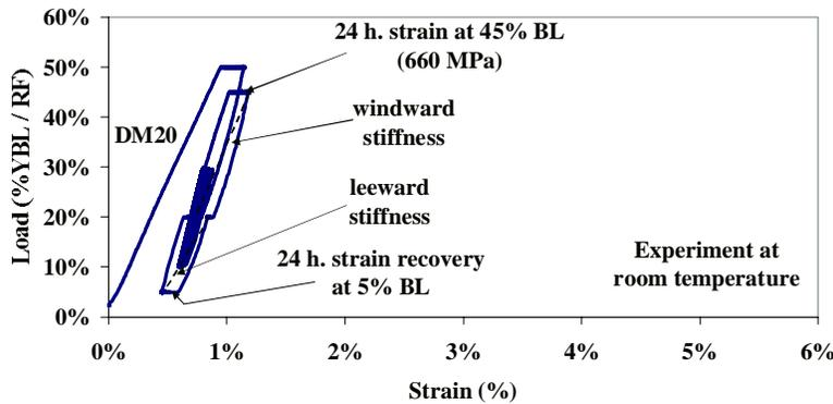
Figure 9. Load – strain results on DM20 fiber at room temperature, based on typical rope application realization factor
