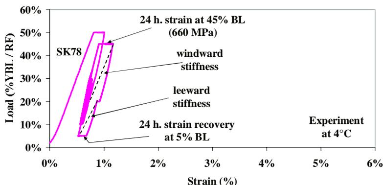
Figure 12. Load – strain results on SK78 fiber at 4°C, based on typical rope application realization factor
