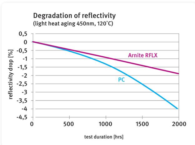
Accelerated light/heat aging test results for Arnite RFLX
