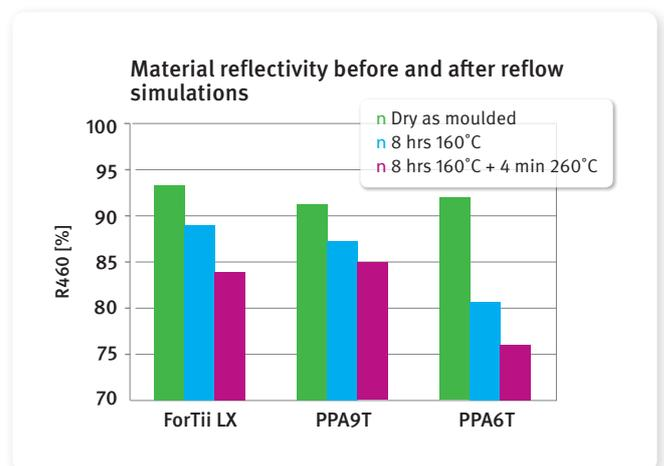
Its high flow properties make it suitable for use in tools with over hundred cavities, and its excellent reflectivity has an immediate positive effect on the light output of the LED package, enabling LED suppliers to improve their key specifications.
