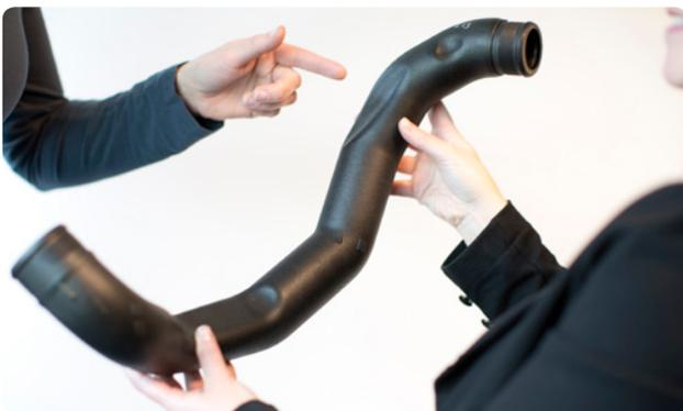
The material was developed to answer the needs of the automotive market, where new EU legislation has set stringent emission reduction targets for 2015. This has led to a trend in smaller vehicles with downsized engines. Creating these smaller engines requires new part designs. For air ducts, neither metal nor injection molding offer the design flexibility needed to fit complex under-the-hood
