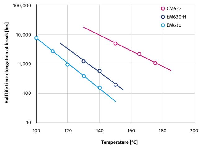
Figure 3 — Comparing the effect of adding a stabilizer and improving the intrinsic stability of the polymer backbone on retention of properties
