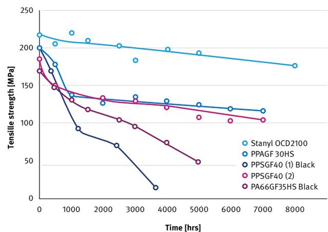
**Figure 5** — Tensile strength retention of Stanyl Diablo versus other materials
