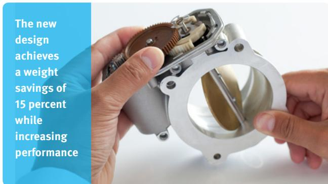
The new design achieves a weight savings of 15 percent while increasing performance, allows for a hood line of up to 5 millimeters lower to save fuel due to less resistance, and delivers a two-year gain in service lifetime to five. The new electronic throttle body, which entered the market in 2010 model year vehicles, meets all interface and performance requirements for all engine management systems, and will replace all existing gasoline and diesel actuators in GM vehicles by 2015.
