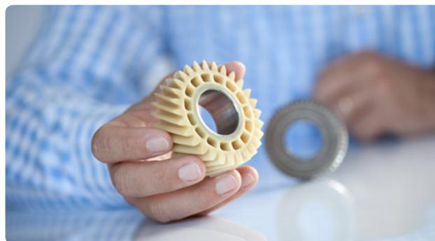
DSM's Stanyl® polyamide 46 (PA46) is one of the main polymers used in under the hood automotive applications due to its superior mechanical and tribological properties. With a melting point of 295°C, this high-performance material has been engineered to retain its mechanical properties at temperatures ranging from 100 to 170°C.
