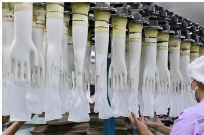
*ForTii Care can replace metal and ceramics used to manufacture medical rubber gloves, reducing operating costs and environmental impacts from manufacturing.*
