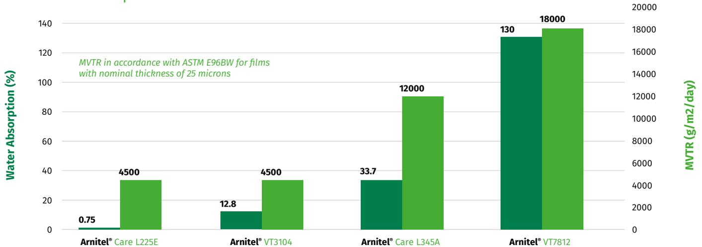
A key measurement of breathability is the Moisture Vapor Transmission Rate (MVTR) – a test that assesses material permeability to water vapor. Requirements for MVTR, water absorption, gas permeation to oxygen, and membrane flexibility and softness vary from application to application. Thanks to Arnitel Care and Arnitel VT's versatile chemistry, membranes can be designed to meet a wide range of property requirements that can't be achieved through microporous membranes.
