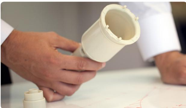
With more than 25 years of experience supplying a special grade of Arnite material for precision safety components, DSM leads the market for brake booster valve bodies. The brake booster valve body amplifies the braking force, making it the heart of the braking system. It is crucial that it operates reliably and faultlessly for the lifetime of the vehicle. For this application, Arnite is the industry
