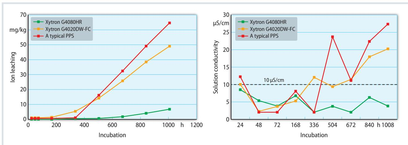
**Fig. 2.** Xytron G4080HR has the lowest ion leaching (left) and solution conductivity (right) compared to other 40% glass fiber-reinforced PPS connections. A solution conductivity of  $10\ \mu\text{S}/\text{cm}$  as an indication of low ion leaching is considered the ideal level to ensure a long cell life
