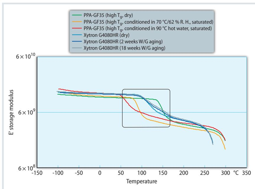
**Fig. 4.** Comparison of the DMTA storage modulus (elastic modulus) between PPA with high  $T_g$  and PPS at different stages (dry as molded, after moisture absorption until saturation and after hydrolytic aging; W/G = water/glycol). Source: DSM; graphic: © Hanser
