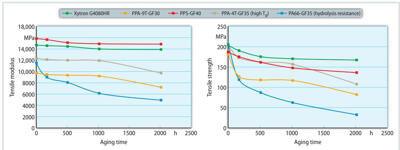
**Fig. 3.** Comparison of the tensile modulus (left) and the tensile strength (right) of different polymer compounds: the aging resistance of the two PPS compounds is higher than that of the PA and the two PPA. Source: DSM; graphic: © Hanser
