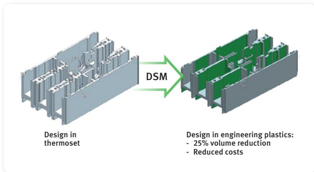
Fig.2 Optimized design of MCCB housing
