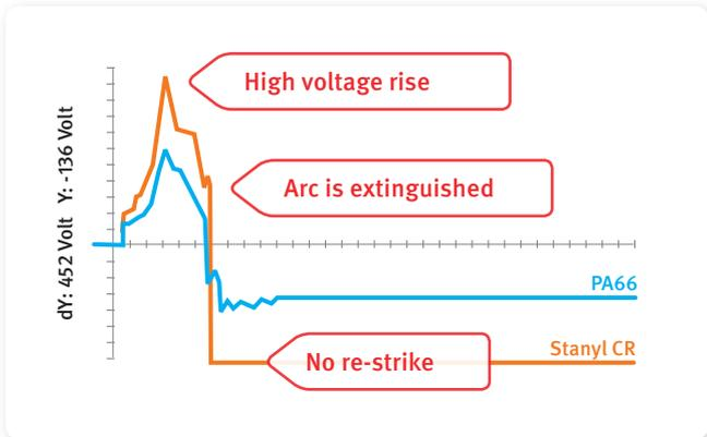
Fig.4 Arc quenching performance
