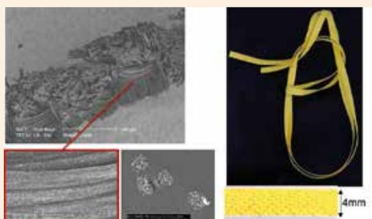
Figure 2 [Right]: 4mm-wide radiopaque UHMWPE sublaminar wire and the double-loop sliding knot with extra pass used to secure the wire. [Left]: Scanning Electron Microscope clearly show homogeneous distribution of Bismuth Tri-oxide (20% weight addition) particles used as radiopacifier.
