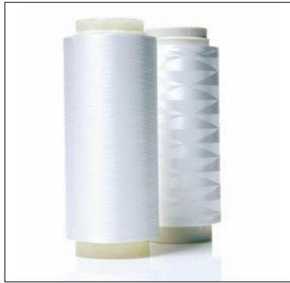
Fig. 3 — Examples of UHMWPE fibers.
