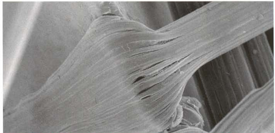
SEM picture of UHMWPE fibre filament stretched over the sharp edge of a razorblade, demonstrating the increased contact surface and high compliance.
