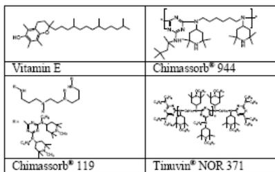
Fig. 1. Chemical structure of used stabilizers
