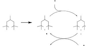
Scheme 1. Simplified radical scavenging mechanism of HALS Stabilizers
