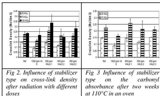
Fig 2. Influence of stabilizer type on cross-link density after radiation with different doses
