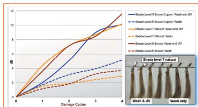
Figure 1. Colour fading curve for natural / auburn colorations under the influence of hand-washing and/or UV irradiation. One damage cycle: 5x hand-washing, drying, conditioning in climate chamber, with or without UV irradiation.
