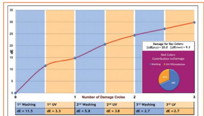
**Figure 4.** Colour fading curve for shade level 3 red colour. Washing with ultrasonic bath and UV irradiation. Particularly noticeable in the two experiments illustrated in Figures 3 and 4 is that the colour fading impact caused by washing diminishes steadily, while the impact of light exposure remains roughly constant. This effect seems to be independent of colour tone.
