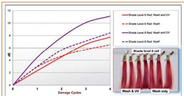
**Figure 2.** Colour fading curve for red colourations under the influence of hand-washing and/or UV irradiation. One damage cycle: 5x hand-washing, drying, conditioning in climate chamber, with or without UV irradiation.
