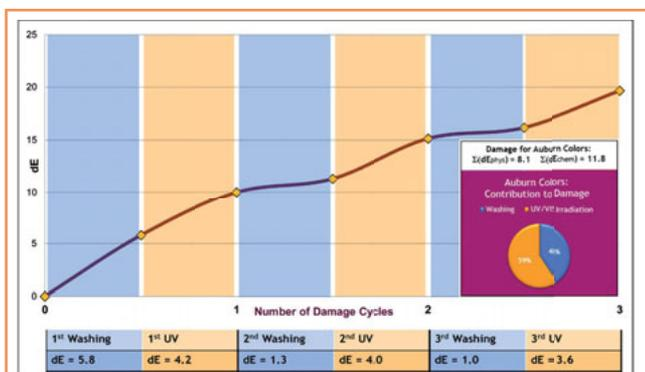
**Figure 3.** Colour fading curve for shade level 5 auburn colour. Washing with ultrasonic bath and UV irradiation.
