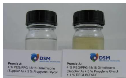
Picture 2 A + B: Premix as recommended above: 4 % PEG/PPG-18/18 Dimethicone (left: Supplier A, right: Supplier B) + 5 % Propylene Glycol + 1 % REGU®-FADE
