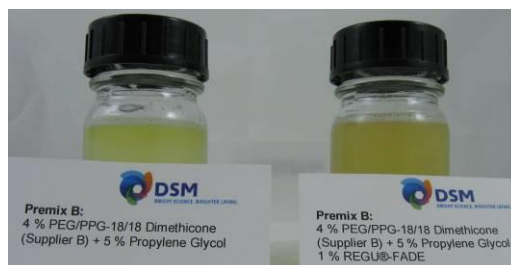
Picture 2 A + B: Premix as recommended above: 4 % PEG/PPG-18/18 Dimethicone (left: Supplier A, right: Supplier B) + 5 % Propylene Glycol + 1 % REGU®-FADE
