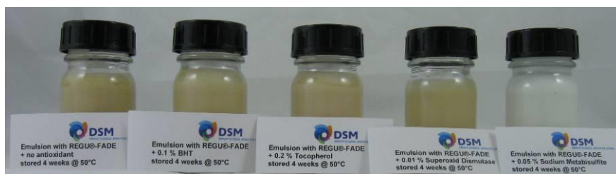
Picture 1: Emulsion with REGU®-FADE + various antioxidants stored @ 50°C for 4 weeks (from left to right: placebo, 0.1 % BHT, 0.2 % Tocopherol, 0.01 % Superoxid Dismutase, 0.05 % Sodium Metabisulfite)
